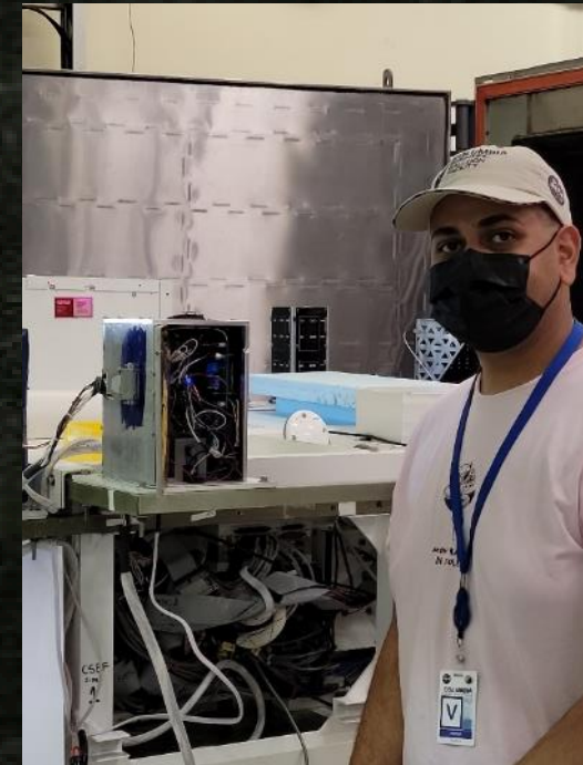
Michael integrating our payload onto the HASP platform, ready for all day thermal/vacuum testing.
